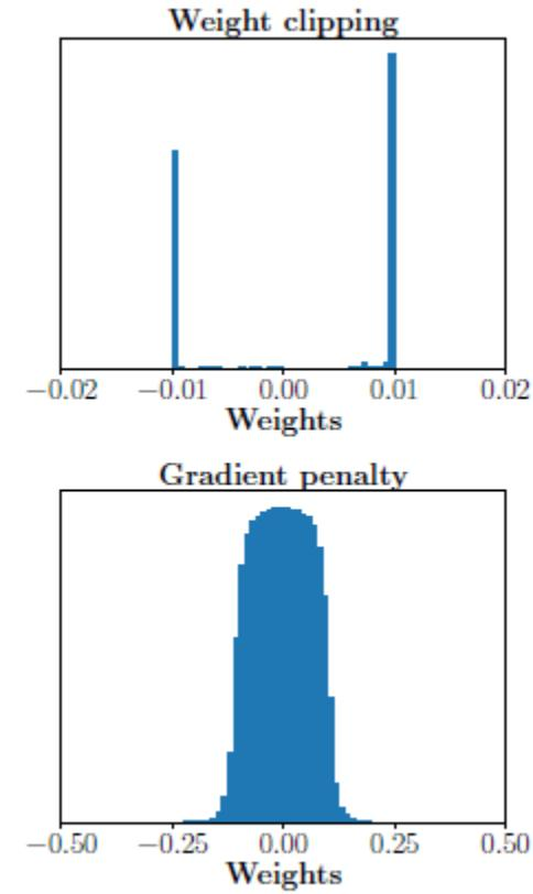
(left) Gradient norms of deep WGAN critics during training on toy datasets either explode or vanish when using weight clipping, but not when using a gradient penalty. (right) Weight clipping (top) pushes weights towards two values (the extremes of the clipping range), unlike gradient penalty (bottom).
