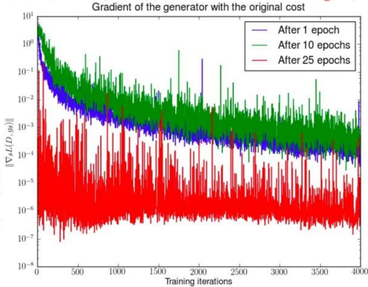
First, we trained a DCGAN for 1, 10 and 25 epochs. Then, with the generator fixed we train a discriminator from scratch and measure the gradients with the original cost function. We see the gradient norms decay quickly, in the best case 5 orders of magnitude after 4000 discriminator iterations. Note the logarithmic scale.
